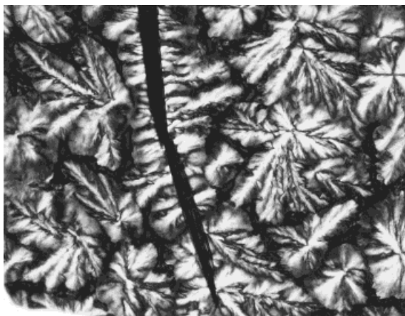
Figure 7 Optical micrographs with crossed polars of bamboo fiber in m -MAPP matrix, showing transcrystalline growth on the bamboo fiber surface ( \times 100 ).
